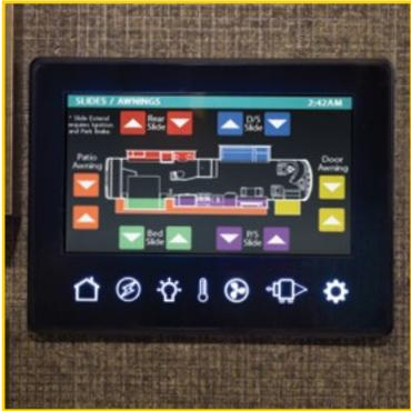
Multiplex Wiring Control System with 7" Touchscreen
