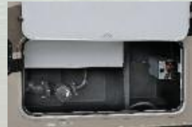
HEATED/ENCLOSED HOLDING TANKS Heated/enclosed utility station uses warm air from the furnace to protect tanks and valves. (N/A 2251 SLE, MBS and Transit)
