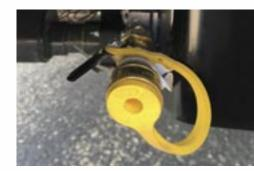
**LP Quick Connect** Each Isata comes with an LP auick connect for use with a portable grill.
