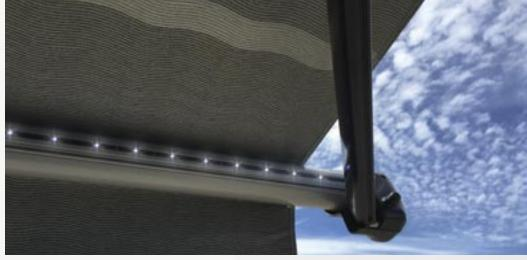
**Power Awning with LED Light Strip** Dual-Pitch, armless awning retracts automatically in high winds.
