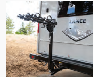
1 1/4" receiver gives you another area to haul your gear including bikes, skis, snowboards, etc. - Limit 130 lbs. - N/A 1475 & 1575
