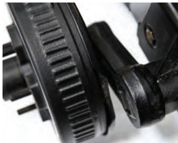
Standard torsion axle provides independent articulation of each tire allowing for a smoother ride.
