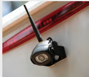
Backup camera w/color display and sound makes backing up a safer, one-person job.
