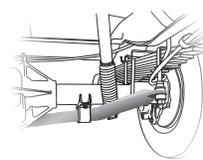
**HEAVY-DUTY REAR STABILIZER BAR** A larger bar and polyurethane bushings, instead of rubber, transfer power faster for extra support, more stability and easier handling
