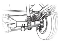
**STANDARD FRONT STABILIZER BAR** Reduces the body roll of a vehicle during cornering or over road irregularities
