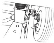
**RUBBER ISOLATION MOUNTS** Positioned near the tires to absorb road shock, dampen noise and minimize vibrations
