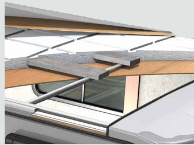
5 1/4" THICK ROOF CROWNED ONE PIECE FIBERGLASS ROOF
