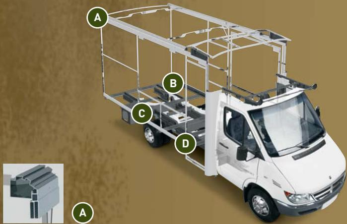
SUPERSTRUCTURE® is the term given to Winnebago Industries' structural motor home design and construction. Rather than a single component, it is the culmination of design integration that incorporates steel and aluminum substructures; welded tubular aluminum floor supports; interlocking joint technology; and Thermo-Panel® floor, roof and sidewalls to form a high-strength, durable vehicle body.
