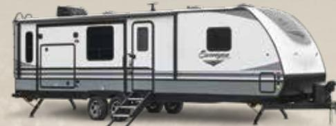
**STRONG, DURABLE LAMINATED FIBERGLASS WITH ALL ALUMINUM CAGE CONSTRUCTION**
