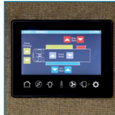
Multiplex Wiring Control System with 7" Touchscreen
