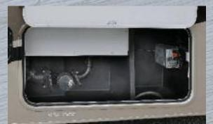
**HEATED AND ENCLOSED HOLDING TANKS** The utility station protects tanks and valves using warm air from the furnace. or damaged power steps. (N/A 2250 SLE, and Transit Series)
