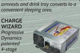
Charge Wizard® converter system can increase battery life by 2 to 3 times or more. It constantly monitors voltage and usage then selects one of four operating modes to properly charge and maintain the battery. Boost, Normal, Storage and Equalization.
