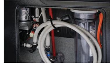
Winterizing tube provides easy access for quick maintenance includes bypass valve. (N/A 2251SLE, 2551DSLE)
