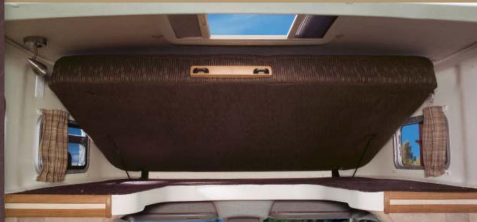
**OVERHEAD BUNK** At night, the bunk provides a spacious and comfortable 49" x 75" sleeping space. Gas struts lift the hinged bunk out of the way during the day for easy cab access.
