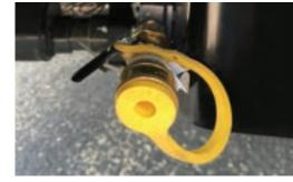
**LP Quick Connect** Each Isata 5 comes with an LP quick connect for use with a portable grill.
