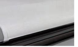
**Fiberglass Roof** This crowned, one-piece, fiberglass roof is more durable and easier to maintain than TPO or rubber.
