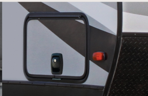
Slam Latch Baggage Doors (Premier only) Durable and convenient, these latches lock with just a slam of the baggage door, providing you with ultimate peace of mind that your valuables are secure.
