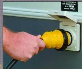
A 30 Amp marine-grade detachable power cord stores in an outside compartment when not in use, saving valuable interior storage space.
