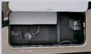
**HEATED AND ENCLOSED HOLDING TANKS**
