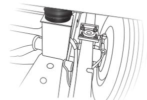
**HEAVY-DUTY REAR STABILIZER BAR** A larger bar and polyurethane bushings, instead of rubber, transfer power faster for extra support, more stability and easier handling
