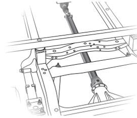
**STANDARD FRONT STABILIZER BAR** Reduces the body roll of a vehicle during cornering or over road irregularities
