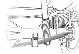
**KONI® SHOCK ABSORBERS** Controls bounce and sway when driving over expansion joints and rough roads
